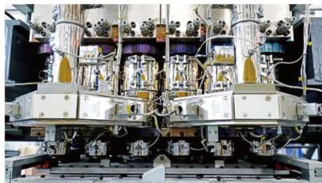
6-Fold ReCo 3-layer Extrusion Head, with View Stripe 3层共挤6模头，带液位线
